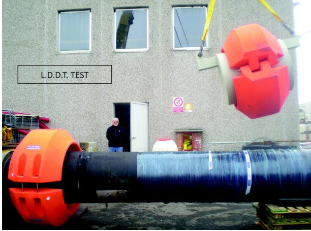
Floatex performed, with positive results, special LDDT (Lateral Dart Drop Test) using two Super Hinged Floats in order to simulate the possible crashes on site and verified the good design of these floats.
